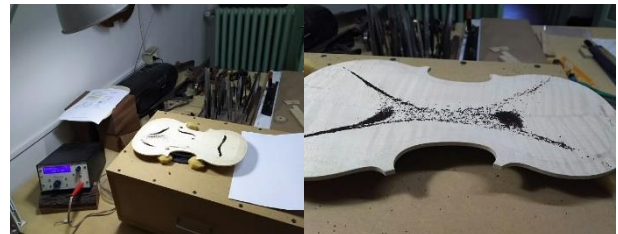
Fig.1 Vibration mode by Chladni method (right: back plate, mode 2)
