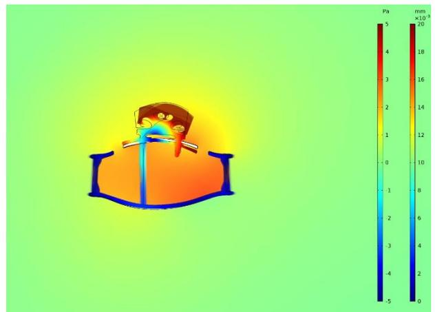
Fig.9 Sound pressure field in y-z plane in forced vibration by sine wave of 196Hz at the G string position on bridge.
