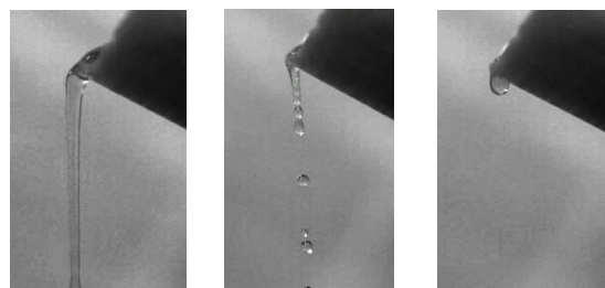
Fig.6 Adhesion of water drop on rectangular edge without channel, setting angle = 30 degree.
