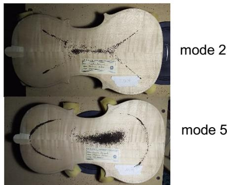
Fig.4 Mode shapes (mode 2, 171 Hz, and mode 5, 352 Hz) of back-plate of violin by Chladni Method.
