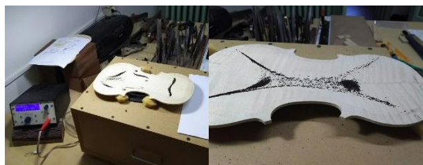
図 9 Vibration mode by Chladni method(mode 2)
