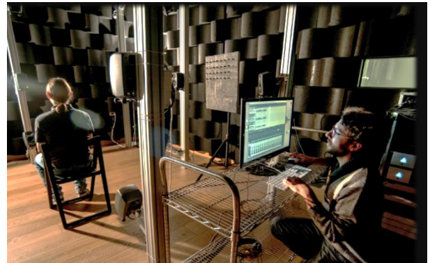
図2 3D audio Rendering at semi-anechoic room (Politechnico di Milano, Musical Acoustic Lab)
