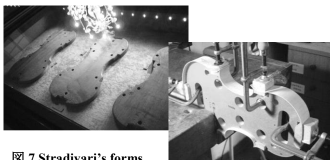
図 7 Stradivari's forms. Ribs and blocks on inside-style form (author's).
