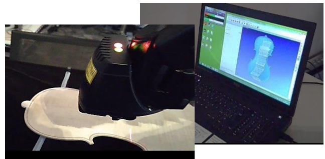
図1 Scanning violin surface by 3D scanner
